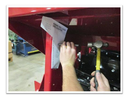
3) Drill holes in the punched locations. Repeat for other side of adapter.
