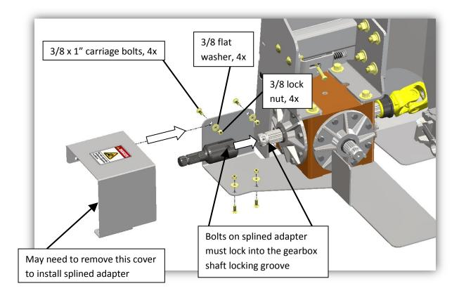
2. If needed, attach the splined adapter to the Claas adapter as shown below:
