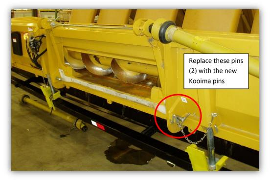
If you have a 12-row head, replace your left side PTO on the head (circled below) with the new one purchased from Kooima, part number KLEX12LEFT. This PTO shaft will connect from the head to the adapter gearbox.
