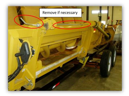
7. Pick up corn header with adapter and cutter. If necessary, loosen bolts and adjust pin connector plates for better pin fit. Attach PTO shafts to adapter and forage harvester.
