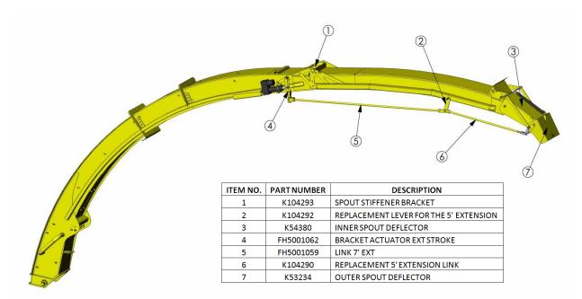
Figure 1: Correctly Installed Extension with Parts Breakdown
