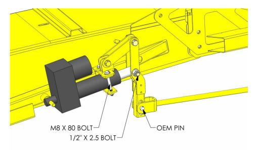
Figure 2: Actuator Mechanism Hardware
