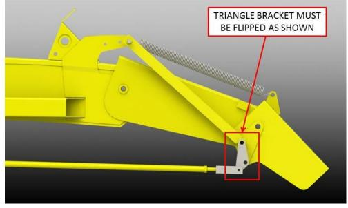
Figure 4: New Bracket Position
