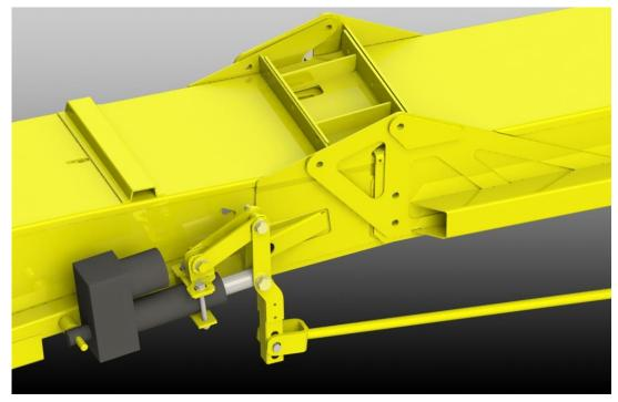
Figure 3: Actuator Mechanism Installed On Spout
