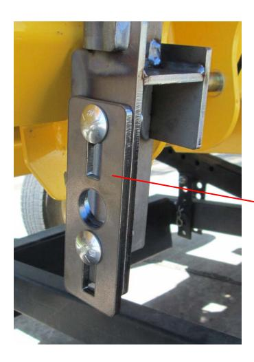
Adjust this plate as needed for proper fitup to forage harvester
