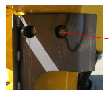
Loosely install the M12 bolts and washers into the side of the head frame as shown. The oversized holes in the guide plate are for socket clearance to access the bolt head.
