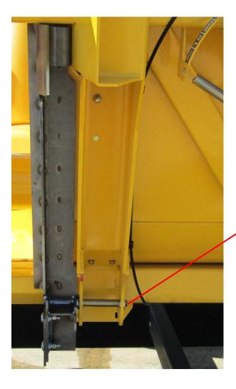
Re-install the M12 bolt, washers, and sleeve saved from the first step. Tighten with the included new lock nut making sure the adapter is sealed as close to the head floor as possible. Tighten the bolts (2) in the previous step.
