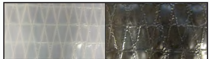
Detail of reinforced string tarps
