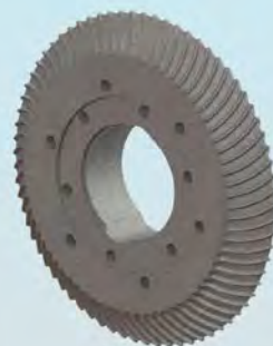
Disc wear after 190,000 tons of silage
